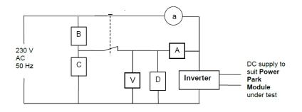
With the unit delivering rated output to resonant load "D", current through ammeter "a" is measured to be zero. After that, the changeover switch is activated, and the unit is connected to the reduced voltage caused by loads "B" and "C". After the changeover switch is activated, the unit is expected to disconnect in less than 1 second. Voltage and current values through time are measured from voltmeter and ammeter "V" and "A" in the diagram above.
